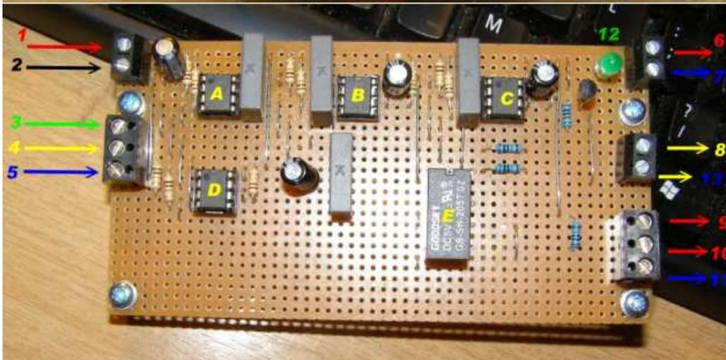
Ideal for making 'breakout boards' or joystick button Matrix boards. The top image shows some Matrix Boards I made for a friend using a BU0836 standard board which required diodes for the permanently on switches (R) and one for the momentary on switches (L) which did not require diodes.
