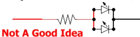
Never connect two LED's up in parallel. It's going to give you problems. Usually the lower value LED only will light. Always connect multiple LED's in series.
